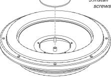
Warning: The dustcap is a structural part of the GTR TunableRadiator™ and must be installed before use.
